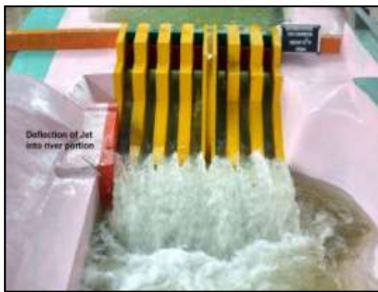
Photo 14: Flow Conditions with deflector wall
